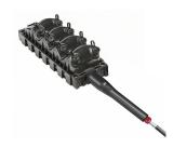
DLX® Mini-MST, Fiber Optic Multiport Service Terminal, 8-port with 1x8 splitter, dielect. flat loose tube cable, Hardened mini-size DLX connector on stub end, 200 m
