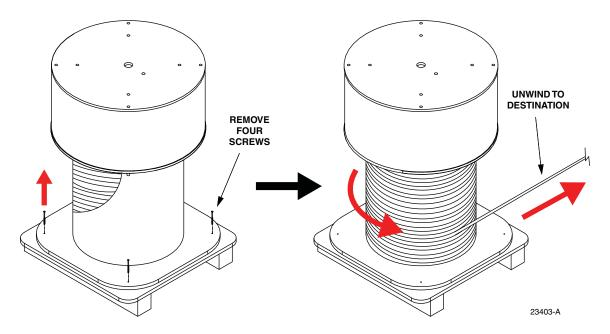
Figure 5. Removing Base Screws and Unwinding Cable
