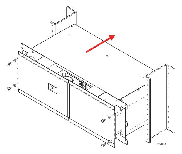
Figure 4. Installing Connector Module on Frame (Cable Not Shown)
