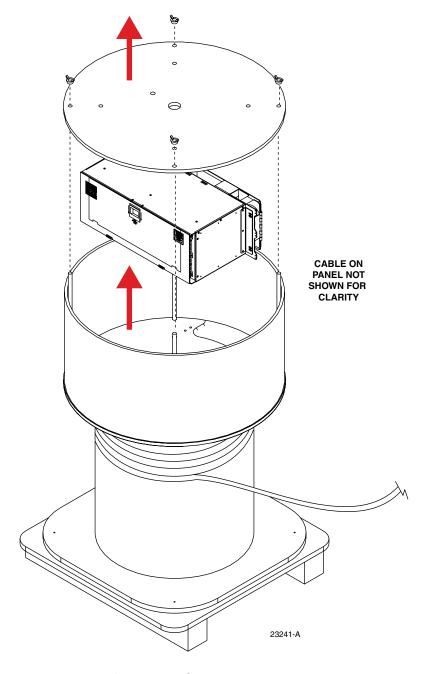
Figure 6. Extracting Connector Module from Hatbox
