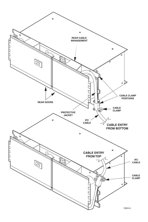
Figure 1. Main Components of Pre-Terminated Rear Load Connector Module
