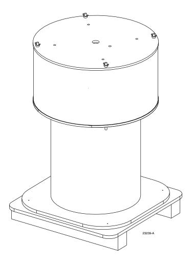
Figure 3. Rear Load Connector Module With Spool
