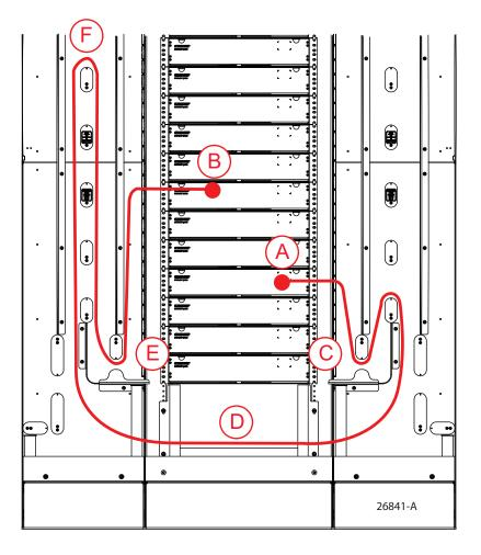
4. **Never** route a patch cord: (A) upward from any panel; (B) in a figure eight pattern; (C) multiple times around the same spool; or (D) directly upward from bottom trough to panel.
