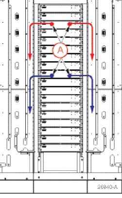
Always store slack on last end to be terminated and terminate both ends before storing slack. To do this: Connect patch cord at first termination point (A). Connect at second termination point (B). Route through vertical cable guide and down and around anchor spool (C). Route through bottom trough (D) to anchor spool (E). Loop over highest storage spool (F), leaving gentle drip loop.
