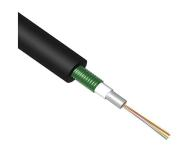
Fiber OSP cable, 6-fiber, OS2, HDPE, loose tube, 6 fiber, gel-filled, Singlemode G.652.D and G.657.A1, 1000 m, Meters jacket marking, Black jacket color
