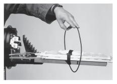
12.3 Place the dome carefully over the trays onto the base. Put the clamp around the base/dome interface. Close the clamp.
