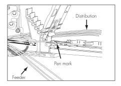
7.5 Secure the transportation tubes to the tray with tie wraps as shown.
