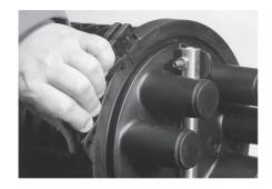
4.2 Open the oval port for cable entry by cutting the port at the ridge with a hacksaw. Deburr the inner edge of the port opening with abrasive strip.
