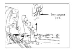
8.2 To remove splice trays from the FOSC-400D base, raise the tray and put the tray support latch down. Pull the tray hinge out of the tray holder bracket, releasing the tray.
