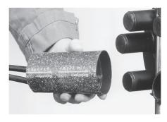
4.4 Slide the cables through the opened oval port. Prepare cables as described in section 5 (cable preparation).
