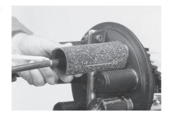
14.9 Match the blue line of the aluminium cable protection foil with the marks on the cables. Wrap the aluminium cable protection foil ground cable.
