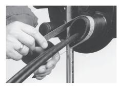
6.3 Place oval seal over the oval port and cable. Mark the sleeve length onto the cable.
