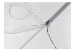
5.3 Cut the loose tube, at a distance of 40 mm from the cable ring cut and remove and degrease fiber bundle. Select a transportation tube which fits over the loose tube. Slip transportation tube over fibers and the loose tube.
