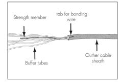
5.2 If a shield continuity is required, cut cable sheath axially for 25 mm from cable ring cut. Crimp shield clip on cable sheath with pair of pliers. Protect the clip with self adhering tape.
