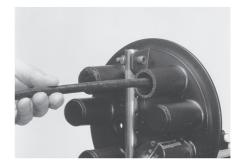
14.5 Align cable ring cut with the edge of the base. Slide strength member into clamp and tighten the nut. Cut away the excess length of strength member.
