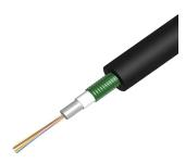
Fiber indoor/outdoor drop cable, LSZH, Gel-filled Central Tube, CST, 6 fiber, Multimode OM4, Meters jacket marking, Black jacket color
