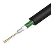
Fiber indoor/outdoor drop cable, LSZH, Gel-filled Central Tube, CST, 6 fiber, Multimode OM3, Meters jacket marking, Black jacket color
