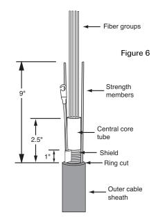
4. If metal shield is present: Remove all but 1" of the metal shield. (Figure 6) Pry open a 1" tab in the exposed metal shield where the shield overlaps. Crimp the bond clamp onto the edge of the shield.
