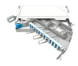
MFPS Fiber Optic panel, 1RU, 48 fibers/RU, splice/patch, SMOUV/front patch cords orientation to the left, 12 SC/UPC, grade C
