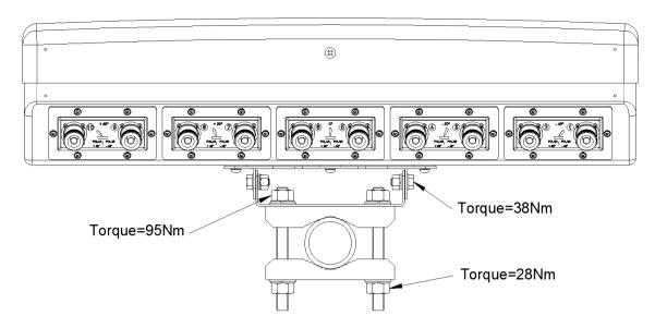
Figure 2. Fixed Downtilt Mounting Bracket Assembled to Antenna & pole
