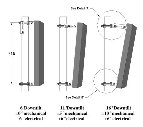
Figure 5. Setting mechanical downtilt
