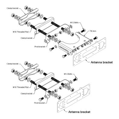
**Figure 4** Arrangement of mounting kits to provide downtilt (details A and B in Figure 5)
