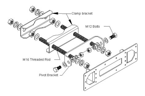
Figure 3. Fixed Downtilt Mounting Bracket Exploded Assembly
