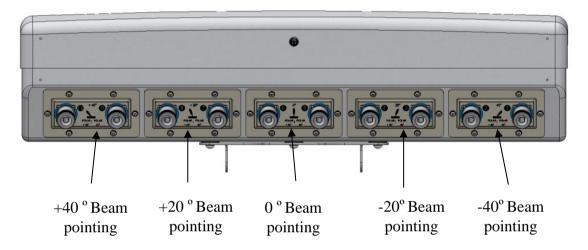
Figure 7 Arrangement of connectors on the base of the antenna.
