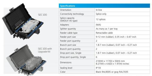
(\*Upgrade kit includes one cover and two additional trays, and increases splice capacity from 12 to 36 splices.)
