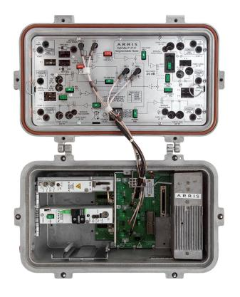
With its premium high-gain receiver and advanced, next-generation GaN hybrid technology, the OM2741 is appropriate for a variety of architectures. The node accepts modules and accessories common with the 4x4 fully segmentable OM4120, easing sparing requirements, reducing inventory, and simplifying deployment training.
