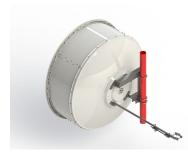
1.8 m | 6 ft ValuLine® High Performance Low Profile Antenna, dualpolarized, 5.925–7.125 GHz, CPR137G, white antenna, flexible woven polymer gray radome without flash, fully assembled/Quick Deploy pack one-piece reflector
