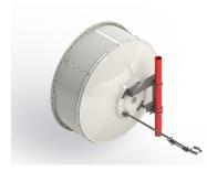
1.8 m | 6 ft ValuLine® High Performance Low Profile Antenna, dualpolarized, 10.000–11.700 GHz, CPR90G, white antenna, flexible woven polymer gray radome without flash, fully assembled/Quick Deploy pack one-piece reflector
