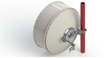
1.2 m | 4 ft ValuLine® High Performance Low Profile Antenna, dual-polarized, 5.925–7.125 GHz, CPR137G, white antenna, flexible woven polymer gray radome without flash, standard pack—one-piece reflector
