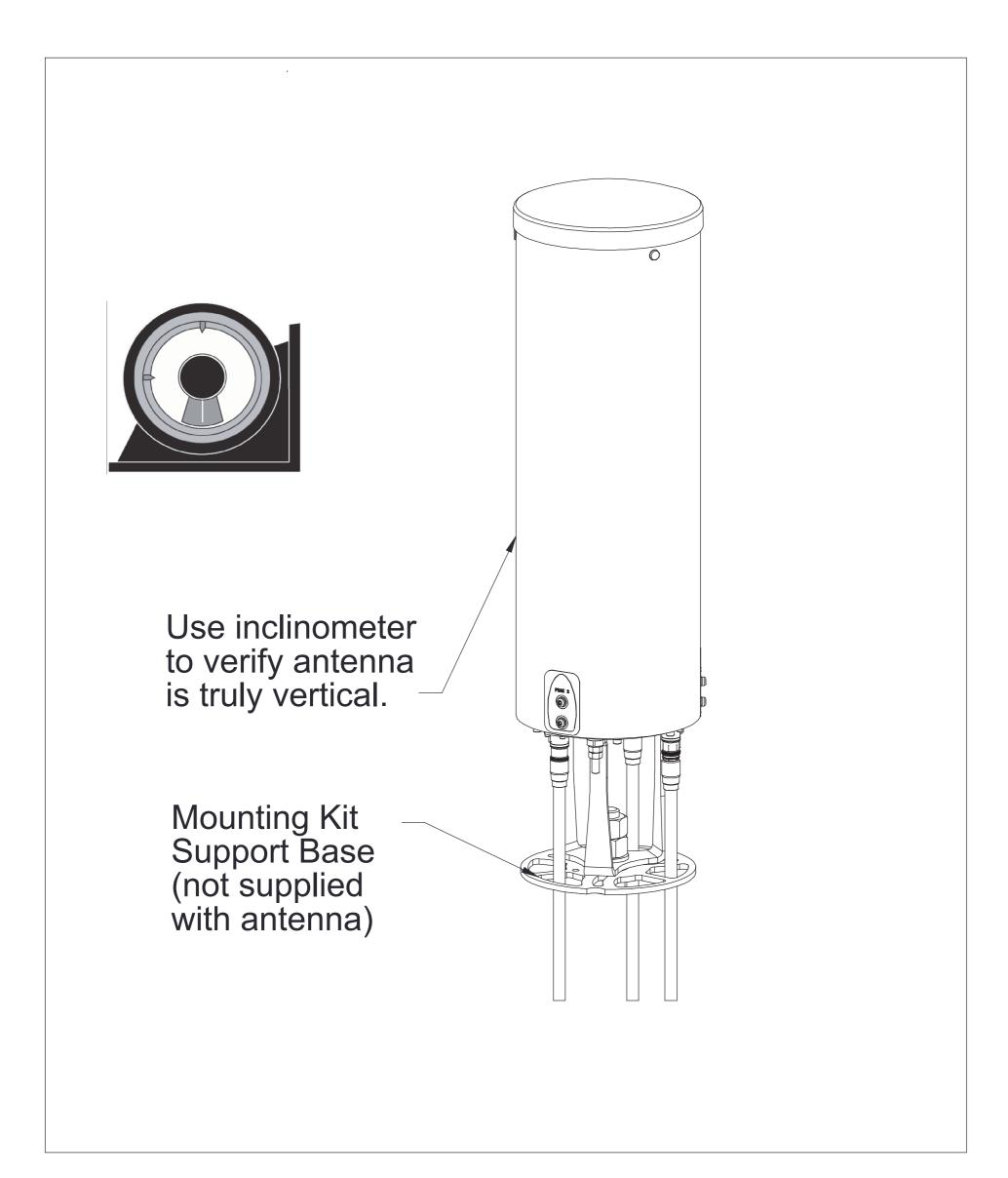
Figure 5. Routing RF Cable and Vertical Alignment
