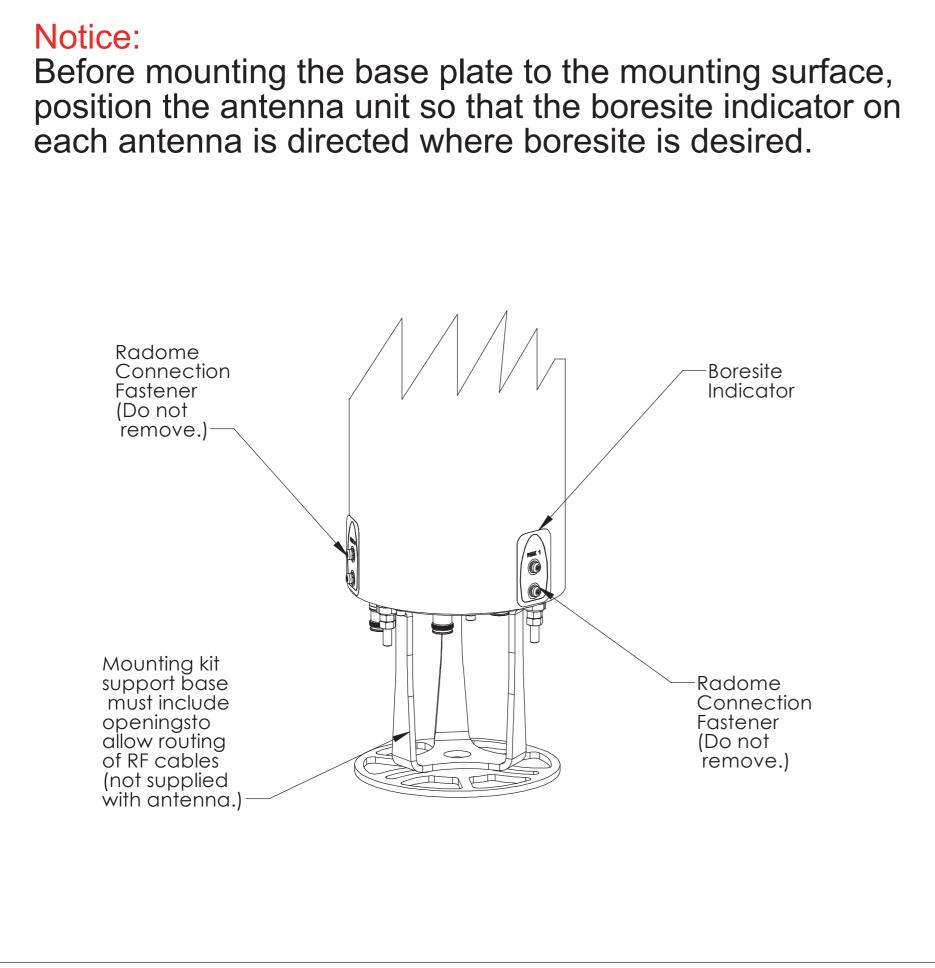
Figure 3. Determining Boresite for Each Antenna.
