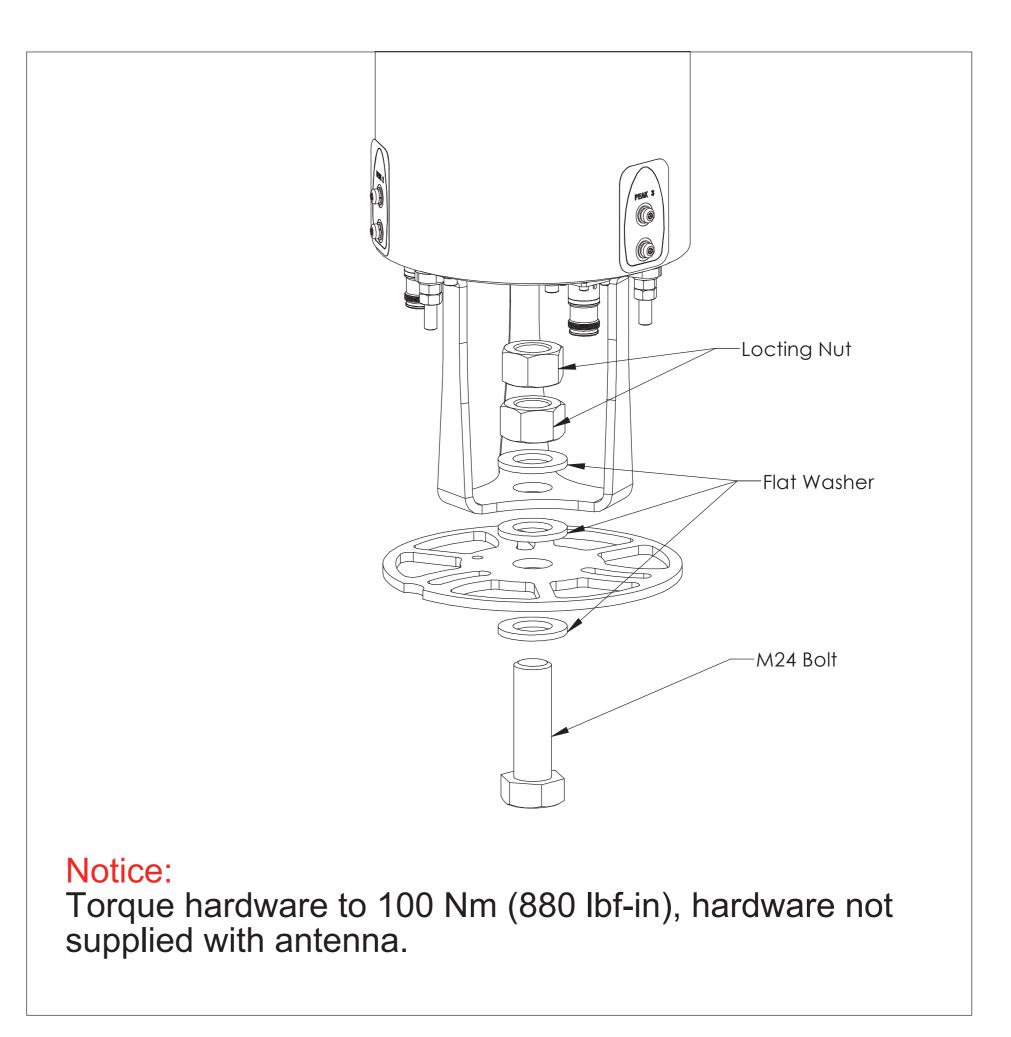
Figure 4. Antenna Installation Interface
