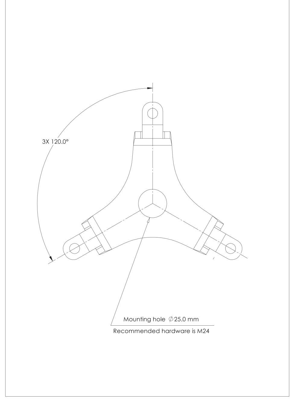
Figure 2. Mounting and Cable Routings Holes on Base.
