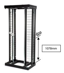
Insert a TF in the outer T-channel (see paragraph 2.2) of each NETpodium back profile at the height of 1078mm measured from the top surface of the NETpodium bottom profile.
