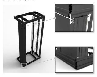
Use an Allan key  $n^\circ 5$  with conical head to fix the side panel with screws and washers (torque of 3.5-4Nm).
