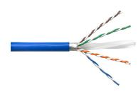
CS41Z3, ETL Verified Category 6A U/UTP Cable, low smoke zero halogen, blue jacket, 4 pair count, 1640 ft (500 m) length reel (EMEA)
