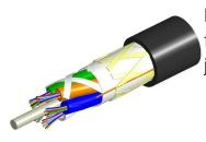
Fiber OSP cable, LightScope® ZWP All-Dielectric Self-Supporting, 144 fiber, 2.5mm Gel-filled Tubes, Singlemode G.652.D and G.657.Al, Feet jacket marking, Black jacket color
