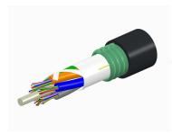
Fiber indoor/outdoor cable, LightScope®, Single Jacket/Single Armor, LSZH, 96 fiber, Gel-filled, Stranded Loose Tube, Singlemode G.652.D and G.657.A1, Meters jacket marking, Black jacket color, Cca flame rating
