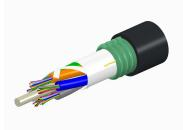
Fiber indoor/outdoor cable, LightScope®, Single Jacket/Single Armor, LSZH, 96 fiber, Gel-filled, Stranded Loose Tube, Singlemode G.652.D and G.657.A1, Meters jacket marking, Black jacket color, Cca flame rating
