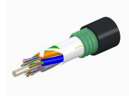
Fiber indoor/outdoor cable, LightSCOPE® Indoor/Outdoor, Single Jacket /Single Armor, Low Smoke Zero Halogen (LSZH), Singlemode G.652.D and G.657.A1, 72 fiber, Gel Filled , Stranded Loose Tube, Feet jacket marking, Black jacket color, Cca flame rating
