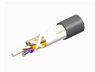
Fiber indoor/outdoor cable, LightScope ZWP®, Single Jacket All-Dielectric, Plenum Rated, Singlemode G.652.D and G.657.Al, 72 fiber, Gel-Free, Stranded Loose Tube, PVDF jacket, Feet jacket marking, Black jacket color
