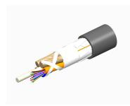
Fiber indoor/outdoor cable, LightScope ZWP®, Single Jacket All-Dielectric, Plenum Rated, Gel-Free, Singlemode G.652.D and G.657.Al, 24 fiber, Stranded Loose Tube, PVDF jacket, Feet jacket marking, Black jacket color
