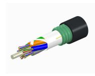
Fiber OSP cable, LightScope ZWP® Single Jacket/Single Armor, 228 fiber, Gel-Free, Stranded Loose Tube, Singlemode G.652.D and G.657.A1, Feet jacket marking, Black jacket color
