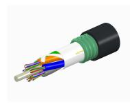
Fiber OSP cable, LightScope ZWP® Single Jacket/Single Armor, 156 fiber, Gel-Free, Stranded Loose Tube, Singlemode G.652.D and G.657.A1, Feet jacket marking, Black jacket color
