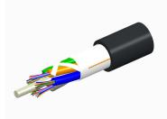
Fiber OSP cable, LightScope ZWP® Single Jacket All-Dielectric, 8 fiber, Gel-Free, Stranded Loose Tube, Singlemode G.652.D and G.657.A1, Meter jacket marking, Black jacket color
