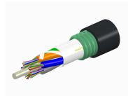
Fiber OSP cable, LightScope ZWP® Single Jacket/Single Armor, 30 fiber, Gel-Free, Stranded Loose Tube, Singlemode G.652.D and G.657.Al, Feet jacket marking, Black jacket color
