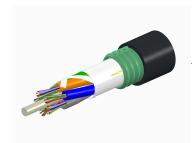
Fiber OSP cable, LightScope ZWP® Single Jacket/Single Armor, 240 fiber, Gel-Free, Stranded Loose Tube, Singlemode G.652.D and G.657.Al, Feet jacket marking, Black jacket color
