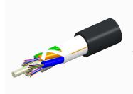
Fiber OSP cable, LightScope ZWP® Single Jacket All-Dielectric, 8 fiber, Gel-Free, Stranded Loose Tube, Singlemode G.652.D and G.657.A1, Feet jacket marking, Black jacket color
