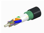
Fiber OSP cable, LightScope ZWP® Single Jacket/Single Armor, 20 fiber, Gel-Free, Stranded Loose Tube, Singlemode G.652.D and G.657.A1, Feet jacket marking, Black jacket color
