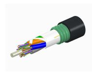
Fiber OSP cable, LightScope ZWP® Single Jacket/Single Armor, 192 fiber, Gel-Free, Stranded Loose Tube, Singlemode G.652.D and G.657.A1, Feet jacket marking, Black jacket color
