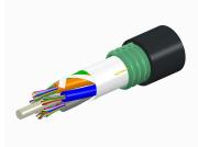
Fiber OSP cable, LightScope ZWP® Single Jacket/Single Armor, 60 fibers, Gel-Free, Stranded Loose Tube, Singlemode G.652.D and G.657.A1, Feet jacket marking, Black jacket color
