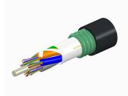
Fiber OSP cable, LightScope ZWP® Single Jacket/Single Armor, Gel-Free, 36 fibers, Stranded Loose Tube, Singlemode G.652.D and G.657.A1, Feet jacket marking, Black jacket color
