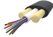
Fiber outdoor drop cable, LightScope ZWP® Self-Supporting All-Dielectric, Singlemode G.652.D and G.657.Al, 8 fiber Arid Core construction, Gel-filled, central loose tube, no ripcords, Feet jacket marking, Black jacket color
