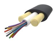
Fiber outdoor drop cable, LightScope ZWP® Self-Supporting All-Dielectric, Singlemode G.652.D and G.657.Al, 4 fiber Arid Core construction, Gel-filled, central loose tube, no ripcords, Feet jacket marking, Black jacket color
