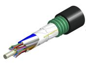
Fiber indoor/outdoor cable, TeraSPEED®, Single Jacket/Single Armor, Low Smoke Zero Halogen (LSZH), 36 fiber, Singlemode G.652.D and G. 657.A1, Gel Filled, Stranded Loose Tube, Black jacket color, Meters jacket marking, Cca flame rating
