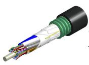
Fiber indoor/outdoor cable, TeraSPEED®, Single Jacket/Single Armor, Low Smoke Zero Halogen (LSZH), 8 fiber, Singlemode G.652.D and G. 657.A1, Gel Filled, Stranded Loose Tube, Meters jacket marking, Black jacket color, B2ca flame rating
