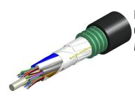
Fiber OSP cable, TeraSPEED® Mini Single Jacket/Single Armor, 24 fiber, Gel-Filled, Stranded Loose Tube, Singlemode G.652.D and G.657.Al, Meters jacket marking, Black jacket color
