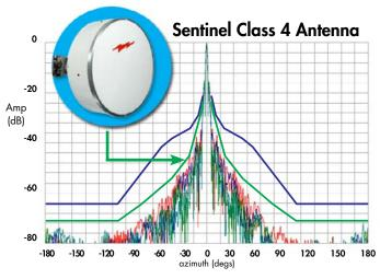
Figure 2: 2 foot 23 GHz measured patterns
