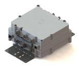
Dual Band Tower Mounted Amplifier, 700//850 MHz, 16 dB, 2 BTS & 4 ANT ports, AISG with 1 RET connector (1 device with 2 sub-units), with 4.3-10 connectors
