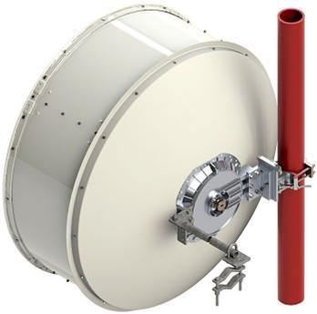
1.2 m | 4 ft Sentinel® High Performance Antenna, dual-polarized, 7.125–8.500 GHz, CPR112G, white antenna, flexible woven polymer gray radome without flash, standard pack—one-piece reflector
