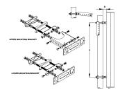
Adjustable Tilt Pipe Mounting Kit for 2.0"-4.5" (60-115mm) OD round members for panel antennas. Includes 2 clamp sets.
