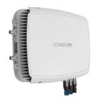
Carrier Access Point with 4-Band Support for Low Power DCS 1800, IMT 2100 and IMT 2600 MIMO Applications, Copper Fed, External DC Powered, with Fan Kit
