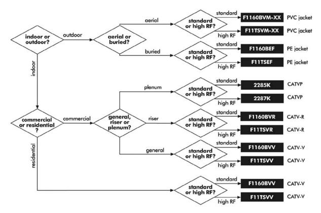
The XX in the part number should be filled with the code for the anti-corrosion agent you'd prefer as follows: **BW** for CommScope's dry BrightWire<sup>®</sup>, or **APD<sup>®</sup>** for the more traditional APD flooding compound. All nonplenum high RF cables are tri-shielded (foil/60 percent braid/ foil); super-shield versions are available. Plenum cables are available only with super-shields.
