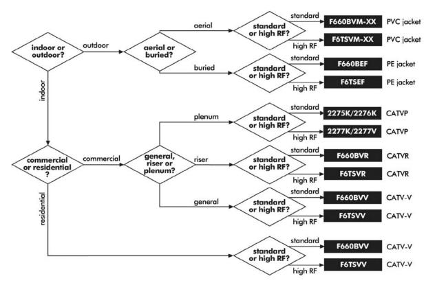
**BW** for CommScope's dry BrightWire<sup>®</sup>, or **APD**<sup>®</sup> for the more traditional APD flooding compound. All nonplenum high RF cables are trishielded (foil/60 percent braid/foil); super-shield versions are available. Plenum cables are available only with super-shields. A 90 percent braid is available for 2276K.
