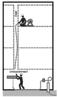
It may be simpler to run the cable on the outside of the building up to each floor or each apartment. A separate cable will be needed for every unit. As always, make a thorough visual inspection of the proposed route and all outlet locations.
