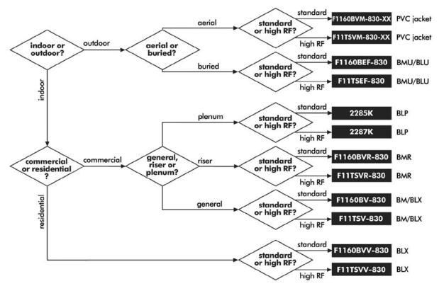
**BW** for CommScope's dry BrightWire<sup>®</sup>, or **APD**<sup>®</sup> for the more traditional APD flooding compound. All nonplenum high RF cables are trishielded (foil/60 percent braid/foil); super-shield versions are available. Plenum cables are available only with super-shields.
