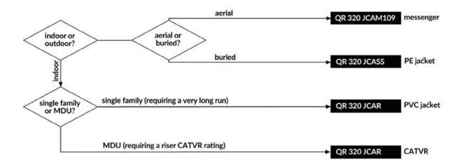
QR 320 cables have a unique welded aluminum strip shield for superior RF protection and a large center conductor for lower attenuation over longer distances. We recommend them for use in MDUs.
