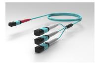
Ultra Low Loss OM4, MPO24 (Unpinned) to MPO8 QSFP (Unpinned), Fiber Extension Cable Assembly, 24-Fiber, Low Smoke Zero Halogen
