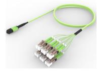
Ultra Low Loss (ULL) OM5 MPO12 (Unpinned) to LC/UPC, Fiber Extension Cable Assembly, 12-Fiber, Plenum
