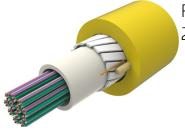
Fiber indoor cable, Plenum All-Dielectric Central Tube Rollable Ribbon, 288 fiber, Singlemode G.657.A2, Feet jacket marking, Yellow jacket color
