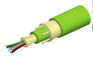
Fiber Indoor Cable, LazrSPEED® Low Smoke Zero Halogen Riser MPO Trunk Cable, 12 fiber, Gel-free, Multimode OM5, B2ca Flame Rating, Feet jacket marking, Lime green jacket color
