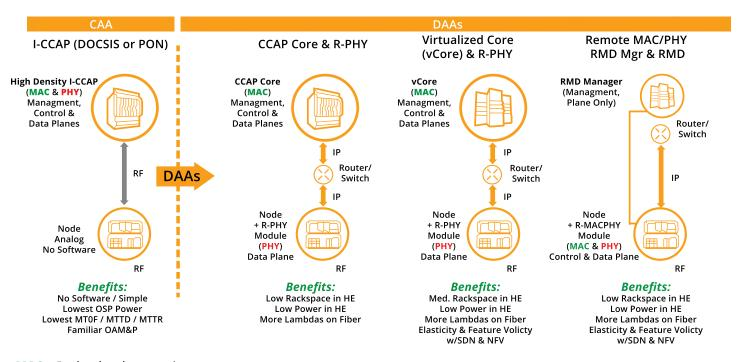
MAC = Packet-level processing PHY = Bit-8F level processing
